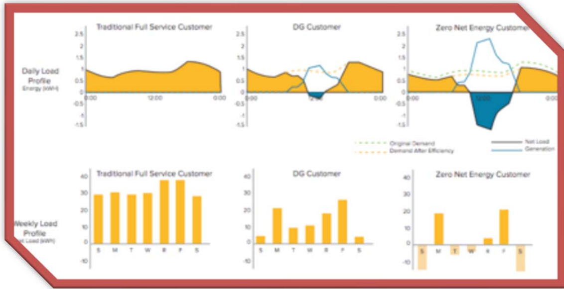
Net Metering is Crucial to Zero Net Energy Buildings (Graphic Courtesy of RMI)
